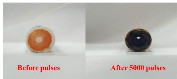
Figure 11: Carbonization of the propellant after pulses
