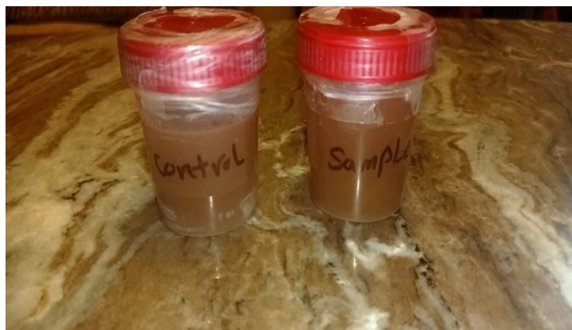
Fig (18): Two samples from the aeration tank :1- pure culture of suspended P. putida (Sample), and 2- negative control culture of wastewater (Control) on 1st Day of incubation.
